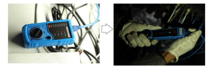
It tests physical connection status of network cable, such as open circuit, short connection, miswire and reverse connection. Operation method
