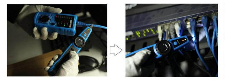
This function is capable of quickly finding the required line pairs among numerous ones. It is adaptable to network cable RJ 45 terminal, telephone line RJ11 terminal. Via an adaptor can test other metal wires. Operation method
