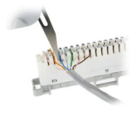
Cut the use of the method: that the cable did not hit the bit or contact bad when you can use a knife to make up!
