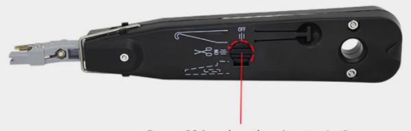
Rotate 90  $^{\circ}$  to close the trimming knife.
