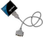
The standard Serial I/O Card features a detachable cable. (CompactFlash card shown.)
