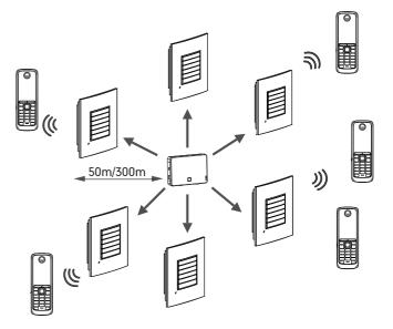
The maximum number of handsets that can be registered to your base station is not affected by the repeater. The repeater can be used to extend the coverage range in all directions, allowing several floors to be covered. The automatic handover process is seamless.
