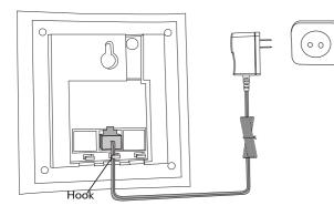
To install the repeater using the supplied screw:
